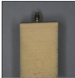
FIGURE 2 - Photograph of a mini-implant inserted in synthetic bone block with 1-mm-thick cortical bone layer.
